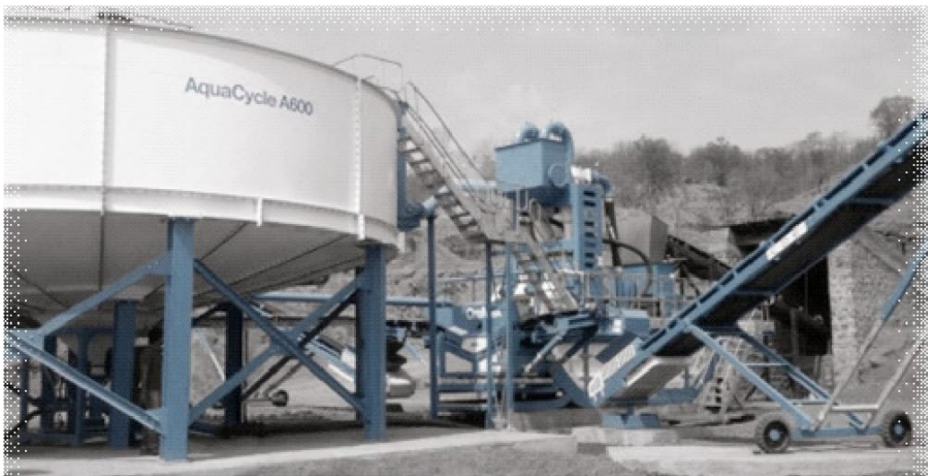
Photo 14: Combo plant for in-situ processing of C&D waste
